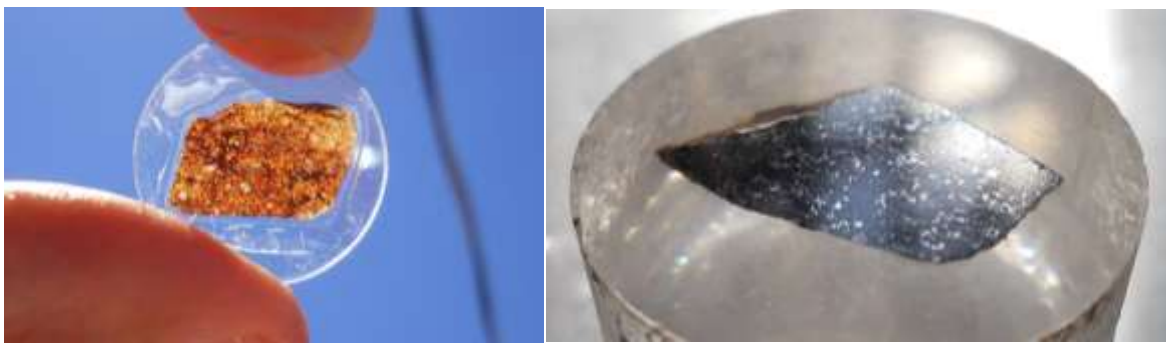
Figure 2 (a) Polished thin section of a meteorite. Polished wafers of samples (typically 30 \mu\text{m} thick) are glued to glass disks.(b) Polished block of meteorite. A sample of material is mounted in a resin block, which is then ground and polished on one surface. The prepared surfaces have a high quality finish that is necessary for a wide range of microscopy and analytical techniques. Images courtesy of Wooddell.
