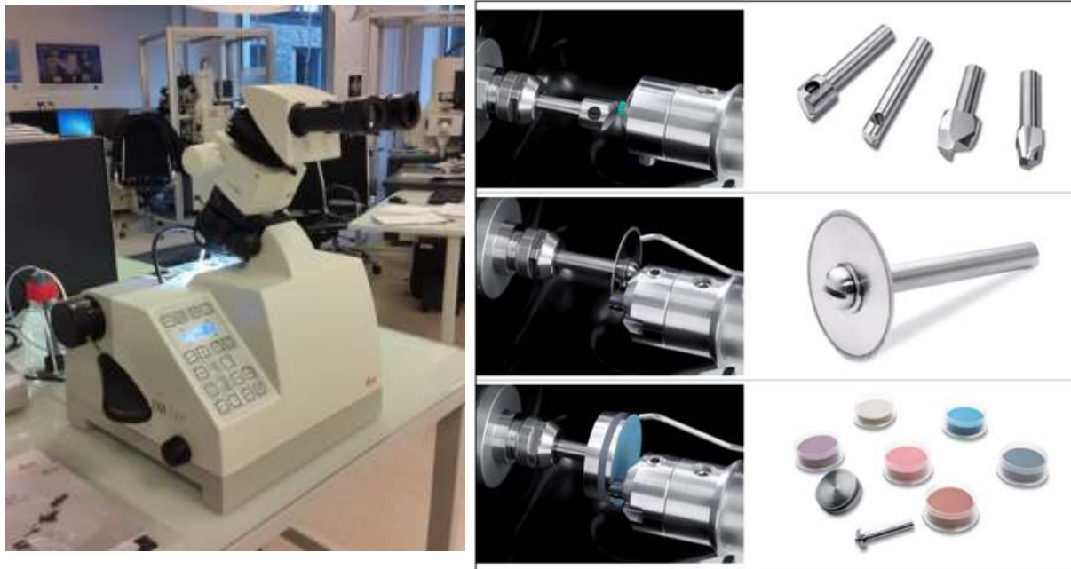
Figure 5 Leica EM TXP sample preparation system for polished mounts (left). On the right are some of the tools used for milling, cutting and polishing.
