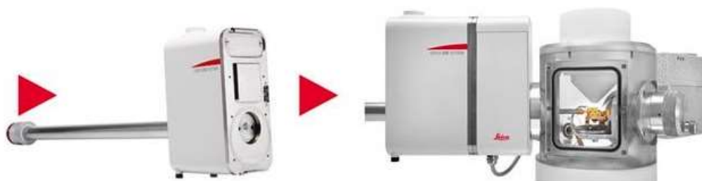
Figure 4 Sample transfer system produced by microscope manufacturer Leica (left) The samples can be loaded into transfer system under clean, inert atmosphere or vacuum conditions. The sample transfer device can then be attached to a compatible docking chamber attached to various compatible instruments and the sample transferred without exposure to unwanted contamination.
